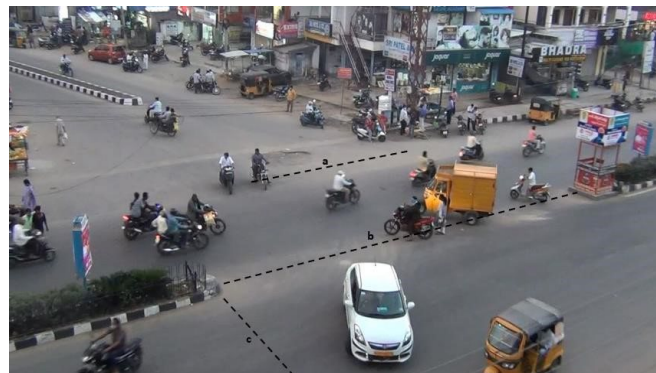
Figure 4: Reference line for right-turning minor traffic
