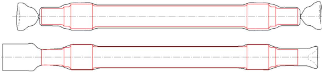
Figure 4: Geometry of a rail axle produced by cross wedge rolling (top) and skew rolling (bottom) with an outline of the finished part
