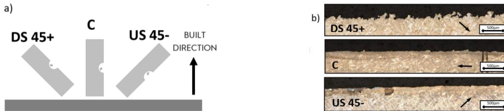
Figure 2: a) Specimen orientation and denomination; b) Surface morphology and near-surface microstructure obtained on etched specimens by LOM
